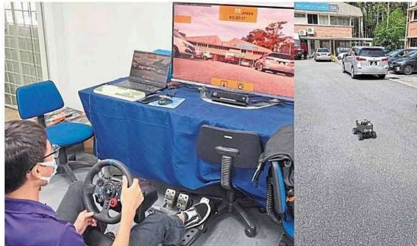
See conducts a live demonstration of the RC car being operated remotely through 5G connection.
